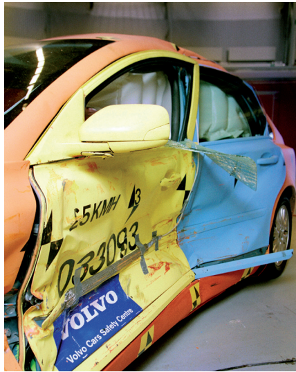
Side impact testing at the US$1 million Volvo Safety Center in Sweden. The deformation, coupled with the deployed airbags, aids passenger safety
