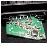
The internal circuit board sensor of the CTS-made accelerator pedal (above left); the internal arms within the pedal caused the voltage to vary as the accelerator was depressed
