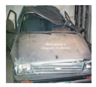
Further aggravating the roof integrity situation are designs that include too many holes, cutouts, notches, dimples, creases, and other discontinuities... plus a minimal number of widely spaced spotwelds, often poorly located along minimal flanges. Because of these needless design defects, the roof is structurally pre-disposed to buckle and collapse.
