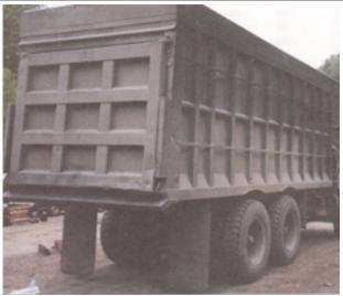
or there is the pretense of a makeshift rear bumper that is totally ineffective. With or without governmental regulations, there is also neglect by truck and trailer manufacturers and operators to voluntarily and compassionately correct the underride hazard by designing and implementing safer trucks and trailers with effective underride prevention guards.
