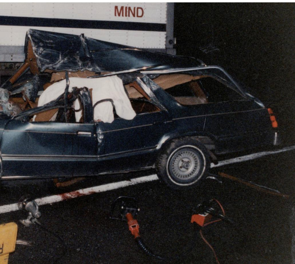
Above and left: In an underride situation, the rigid structures of the taller truck or trailer crash through the windshield, and windshield pillars, ripping and crushing the roof, and penetrating the passenger compartment
